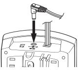
5. Route the modular cord through either groove on the bottom of the base and the adapter cord through the groove below the strain relief slot.
